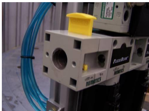
Air shutoff in the operating position (UP)
