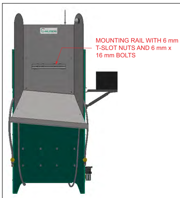
FIGURE 2-3. MOUNTING RAIL LOCATION WITH 6 MM T-SLOT NUTS AND 6 MM X 16 MM BOLTS
