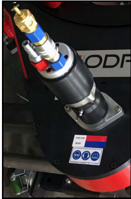
FIGURE 3-14. INSTALLED AIR MOTOR DRIVE
