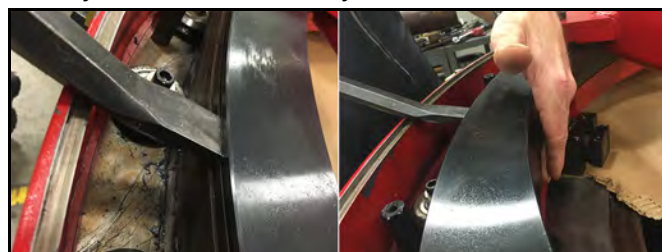
FIGURE 5-6. CHECKING FOR PLAY BETWEEN THE TRACK RING AND THE STATIONARY RING
