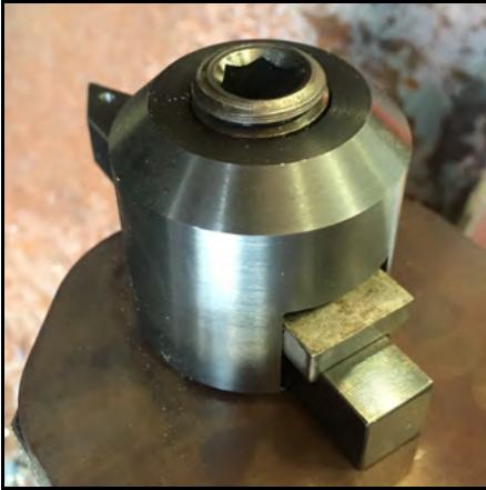
FIGURE 3-10. .50" TOOL ADAPTER INSTALLED (P/N 89175)
