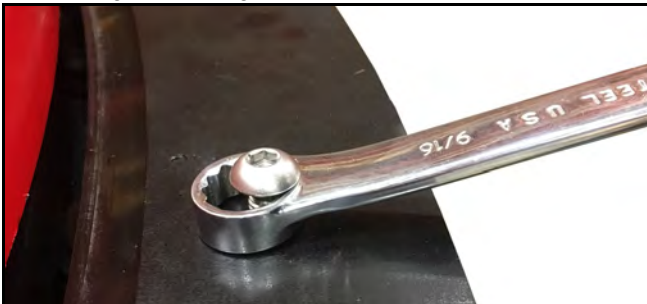
FIGURE 5-2. BOX WRENCH OVER SCREW
