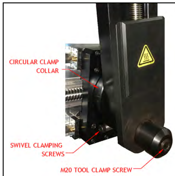
FIGURE 3-9. LOCATION OF SWIVEL CLAMPING SCREW
