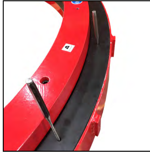
FIGURE 5-3. PUNCHES USED FOR GUARD INSTALLATION
