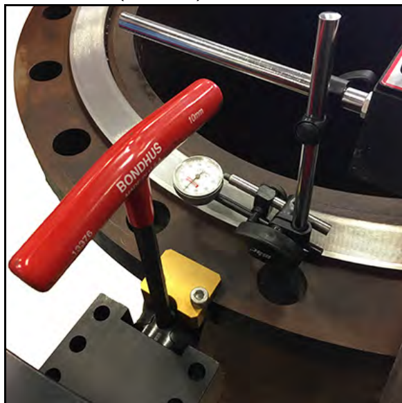
FIGURE 3-8. DIAL INDICATOR MOUNTED FOR LEVELING
