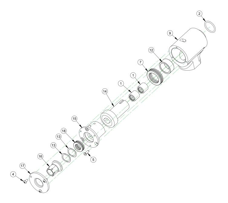
FIGURE A-3. BF-R BOILER GUN BASE UNIT ASSEMBLY 2 (P/N 98894)
