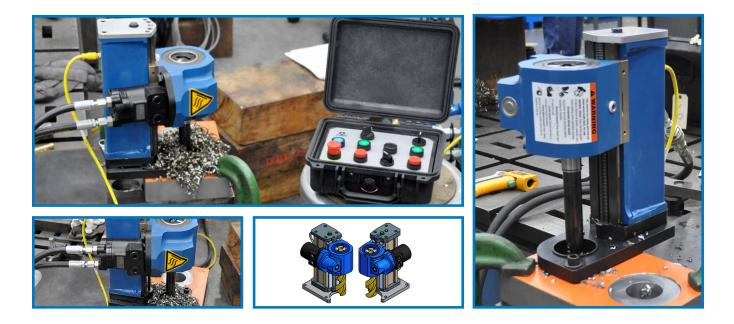
Our family of customizable **Compact Drilling Machines** is ideal for machining applications that call for drilling holes up to 2.5 inches (63.5 mm) in a single pass, step drilling or roto-broaching up to 4.5 inches (114.3 mm) and back-spot facing up to 5.2 inches (132.1 mm). This machine meets tight side clearances which require holes to be within 2.5 inches (63.5 mm) of an obstruction with overhead clearances as low as 15 inches (381 mm).
