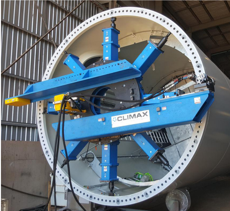
Climax Circular Mill machining a Wind Tower Flange.
