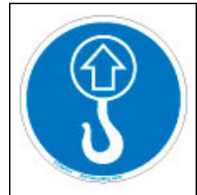
FIGURE 3-1. LIFTING POINT LABEL
