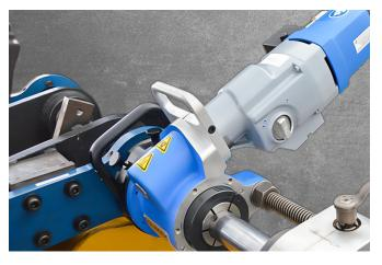
The Eibenstock EAU 34/4 motor has a 4-speed gearbox. For each BB5000 line boring machine setup, select the lowest gear you can (highest motor speed). Try to always run the motor at no lower than 50% of full speed when under heavy loads—the more cooling air passing through the motor, the better.
