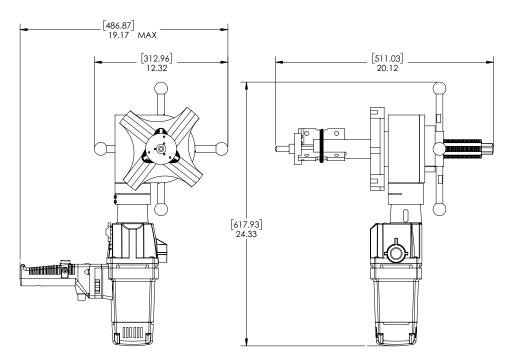
FIGURE 2-5. PB8 POWER BEVELER ELECTRIC DIMENSIONS (P/N PB12EL)
