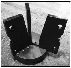
FIGURE 3-1. INSTALLING WEDGE PLATES
