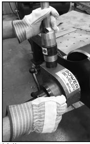
FIGURE 4-1. HAND POSITIONING ON THE PNEUMATIC PB8.
