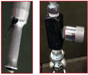
FIGURE 2-2. THROTTLE LEVER (L) FLOW CONTROLS (R)
