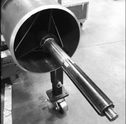
FIGURE 3-6. CENTER SHAFT INSTALLED
