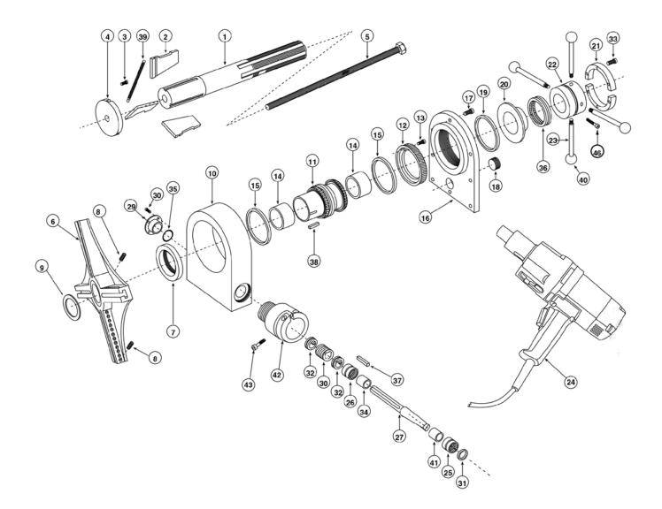
FIGURE A-3. PB8 POWER BEVELER, ELECTRIC ASSEMBLY (P/N PB8EL)
