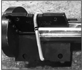
FIGURE 3-3. INSTALLATION OF THE WEDGE GUIDE ASSEMBLY
