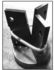
FIGURE 3-2. FITTING AND INSTALLING THE SPRINGS
