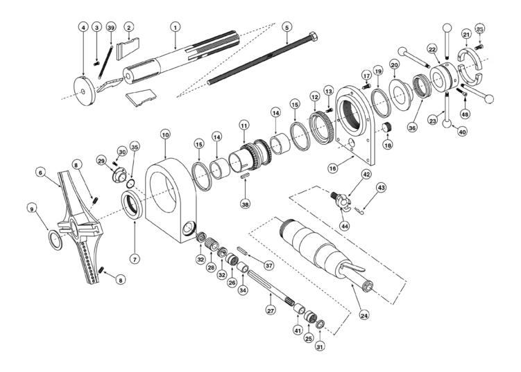
FIGURE A-1. PB8 POWER BEVELER, PNEUMATIC ASSEMBLY (P/N PB8PN)
