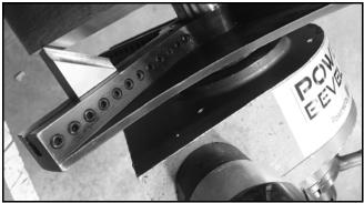
FIGURE 3-7. SINGLE CUTTING BIT INSTALLED
