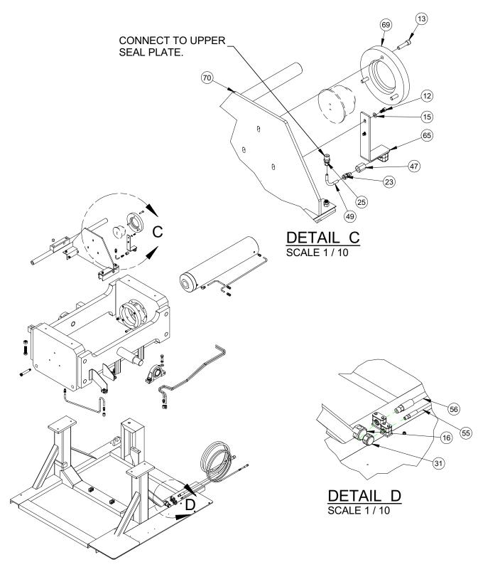
FIGURE A-8. USV-16-200T ASSEMBLY DETAIL C AND D 1 (P/N 91593)
