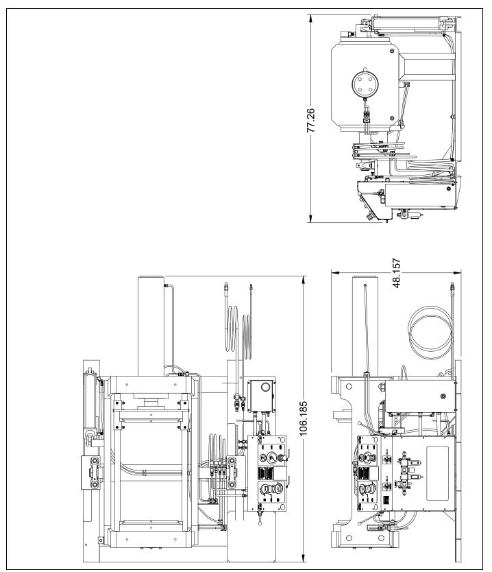
FIGURE 2-4. CLAMP FIXTURE DIMENSIONS
