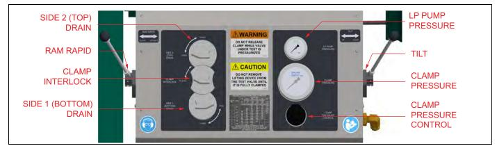
FIGURE 2-2. CONSOLE CONTROLS
