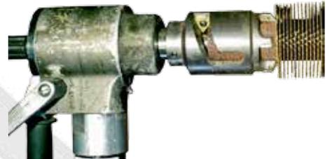
Hand hole cap removal is accomplished with standard tool and cutting head. A special centershaft threads into the cap to lock it securely. Extra wide blades remove the weld without harming the surrounding surface.
