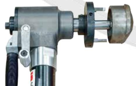
I.D. tracking tool slides are available for several models of tools. They make accurate machining of out-of-round pipes easy and fast.
