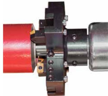
The easy compound bevel. Here our MFT-HD uses power and precision to place a 37.0-10.0° bevel. The unique power enables it to turn formed blades in 9% chrome material. Properly set, the operator merely feeds the blades into the face until a smooth, accurate compound bevel is produced.
