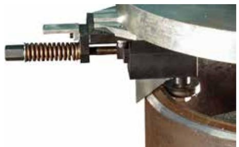
Make short work of stub removal from headers. Here our model MB-110 is equipped with special blades, made to specs, that remove stub weld, chamfer the header and clean up the tube seat in a single pass. Contact us with your specifications to see how easy it is to save time and money.
