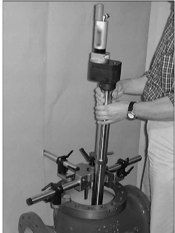
FIGURE 4-19. LOCATING THE MACHINE INTO THE UNIVERSAL CLAMPING DEVICE
