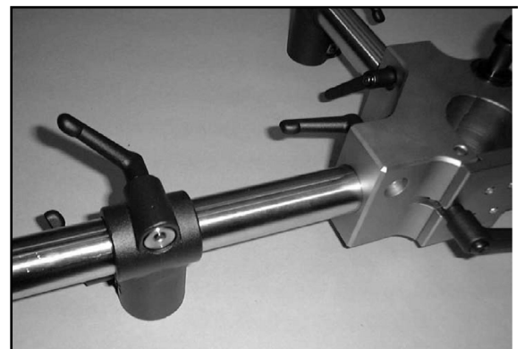
FIGURE 4-5. ASSEMBLY OF ANGULAR CLAMPS ONTO THE SUPPORT PIPES
