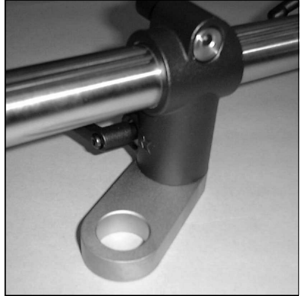
FIGURE 4-6. ASSEMBLY OF CLAMPING SHOES INTO ANGULAR CLAMPS
