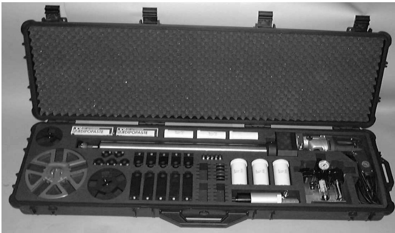
FIGURE 3-1. MACHINE CASE INCLUDING ELECTRIC AND PNEUMATIC DRIVE WITH MAINTENANCE UNIT (VM2350 OPTIONS SHOWN
