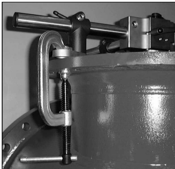
FIGURE 4-9. MOUNTING OF CLAMPING SHOES BY MEANS OF FORGED STEEL CLAMPS
