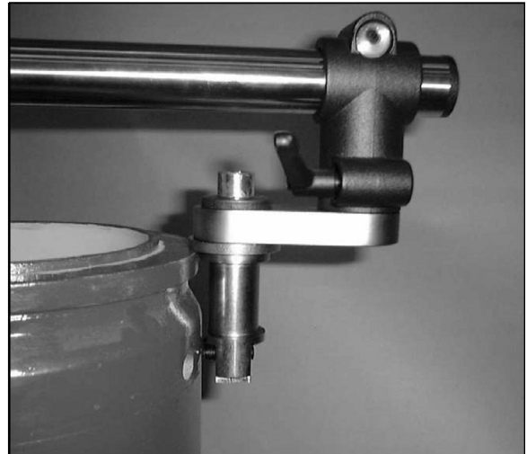
FIGURE 4-10. MOUNTING OF UNIVERSAL CLAMPING DEVICE TO A VALVE BODY WITHOUT FLANGE BY MEANS OF COLLAR BAND SHAFTS (COLLAR BAND IS NOT SHOWN)
