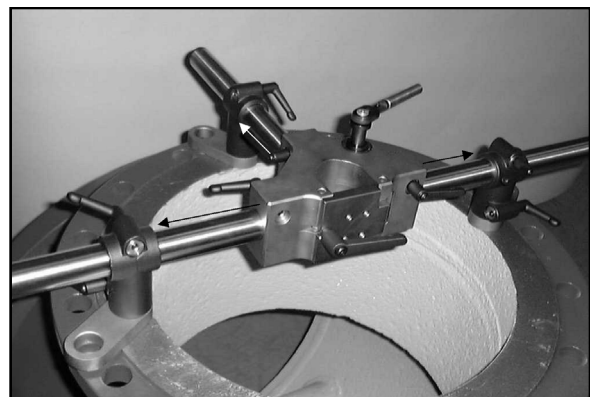
FIGURE 4-7. ALIGNMENT OF THE UNIVERSAL CLAMPING DEVICE
