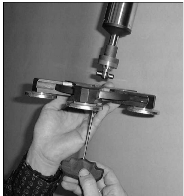
FIGURE 4-16. ADAPTATION OF PLANET WHEEL DIA. 100 MM OR DIA. 135 MM
