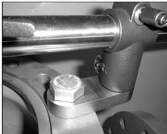
FIGURE 4-8. MOUNTING OF CLAMPING SHOES WITH BOLTS
