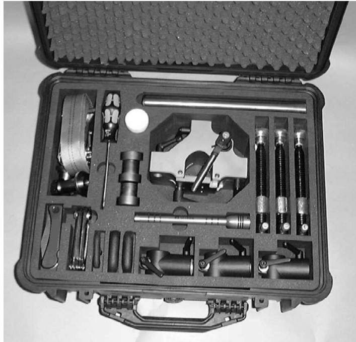
FIGURE 3-2. ACCESSORY CASE WITH UNIVERSAL CLAMPING DEVICE (HERE VM2350)
