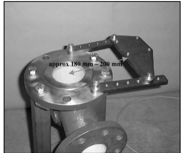
FIGURE 4-7. BRACKETS WITH BASE PLATE MOUNTED ONTO VALVE BODY (FLANGE MOUNTING)
