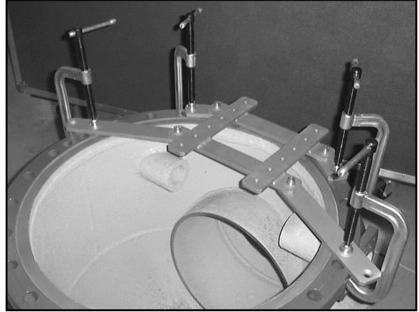
FIGURE 3-10. C-CLAMPS MOUNTING THE BASE TO THE FLANGE
