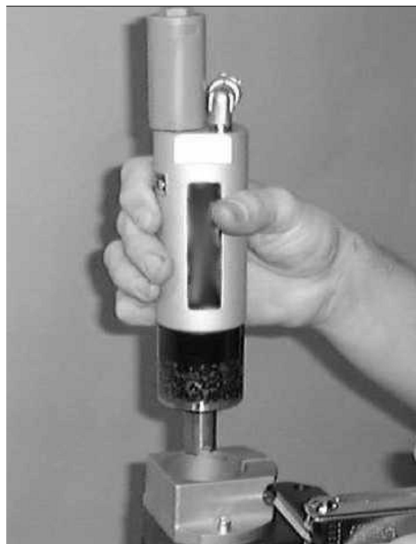
FIGURE 4-5. CHANGE OF MOUNTED DRIVE MOTOR (STANDARD AIR MOTOR SHOWN)
