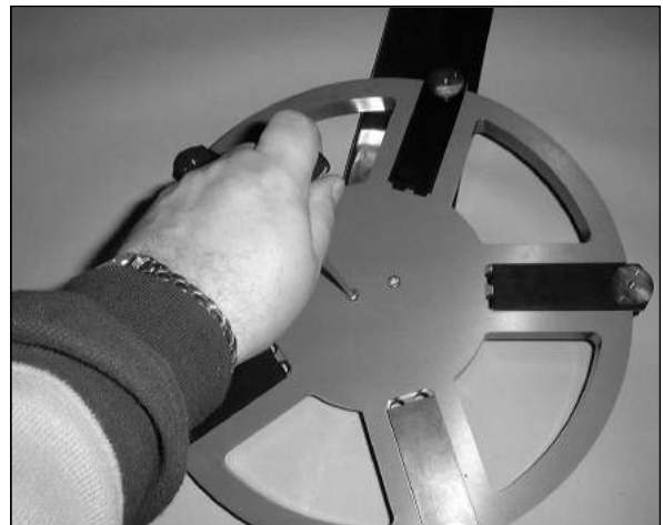
FIGURE 3-14. ADAPTING THE PLANET WHEEL TO BALL JOINT COUPLING
