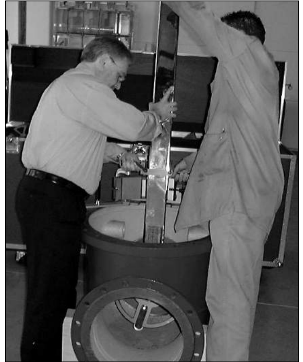
FIGURE 3-15. LOCATING THE MACHINE ARM INTO THE TILTING ADAPTER
