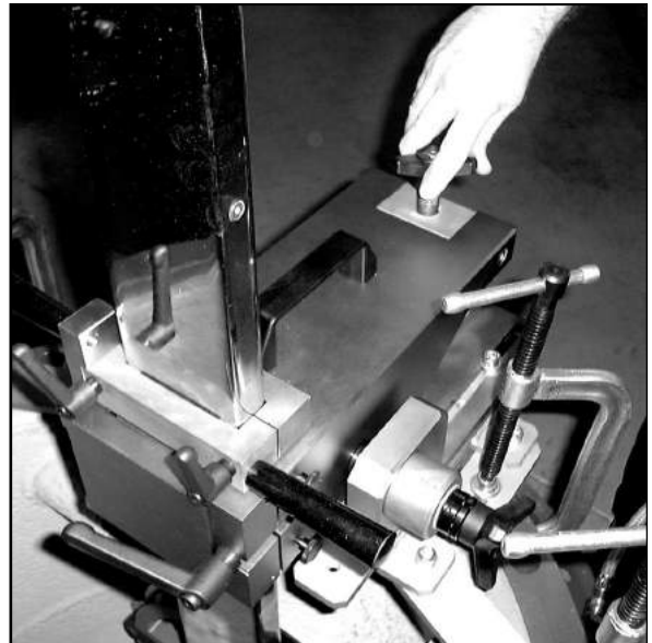
FIGURE 4-1. APPLIANCE OF GRINDING PRESSURE AT STAR KNOB OF TILTING ADAPTER
