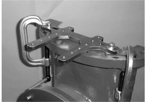
FIGURE 3-10. MOUNTING OF BASE PLATE TO FLANGE BY MEANS OF FORGED STEEL CLAMPS
