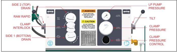
FIGURE 2-2. CONSOLE CONTROLS
