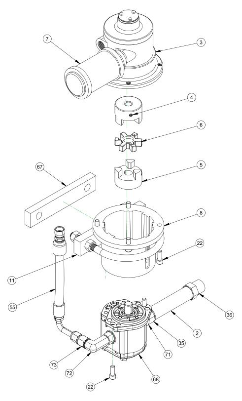
FIGURE A-8. USV-12-150T LP PUMP DETAIL (P/N 87922)
