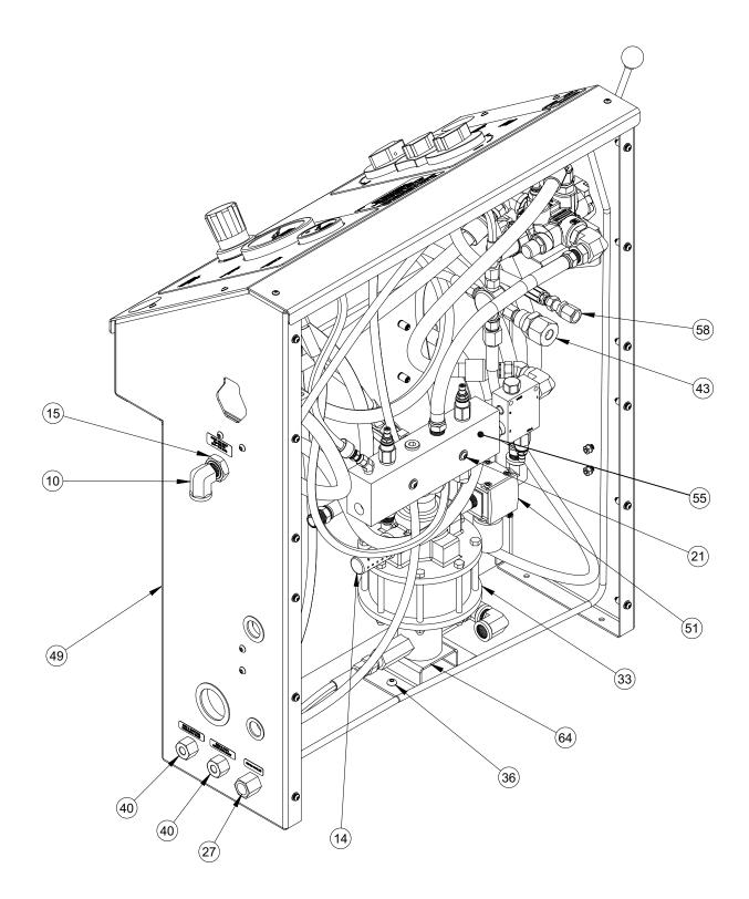
FIGURE A-3. CONTROL CONSOLE USV ASSEMBLY BACK (P/N 89020)
