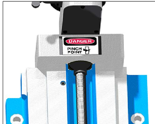
**FIGURE 8 EMPLACEMENT DES ÉTIQUETTES SUR L'ENTRAÎNEMENT D'AVANCEMENT**
