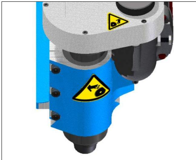
**FIGURE 2 EMLACEMENT DES ETIQUETTES SUR LA BROCHE WELDON**
