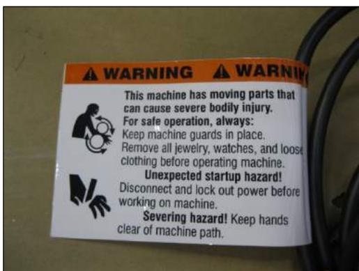
**FIGURE 19 EMBLACEMENT DES ÉTIQUETTES SUR LE CÂBLE ÉLECTRIQUE (ARRIÈRE)**
