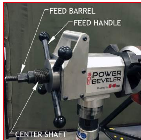
FIGURE 3-3. CUTTING TOOL FEED COMPONENTS
