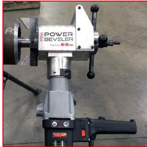
FIGURE 4-2. PB6 WITH ELECTRIC DRIVE MOUNTED ON THE WORKPIECE.
