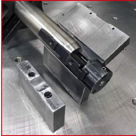
FIGURE 3-1. WEDGE EXTENSION INSTALLATION
