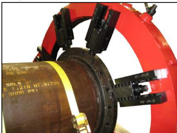
FIGURE 2-1. EXTENSION FEET INSTALLED
