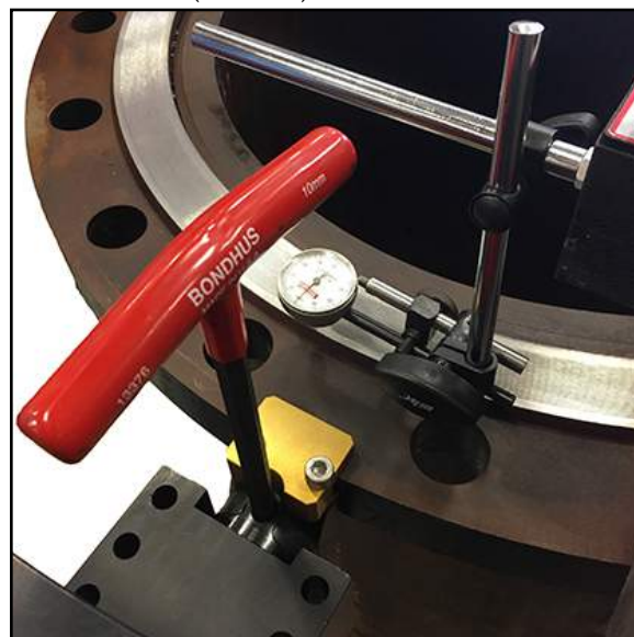
FIGURE 3-8. DIAL INDICATOR MOUNTED FOR LEVELING
