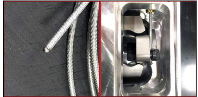
FIGURE 5-11. SOLDER-TREATED CABLE END (LEFT); CABLE END SECURED UNDER THE M4 SCREW (RIGHT)
