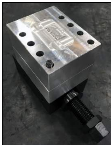
FIGURE 3-7. CHUCK FOOT SPACERS
