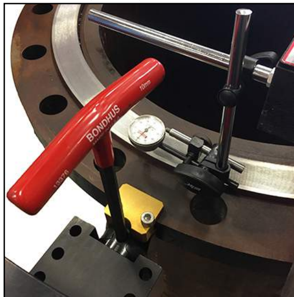
FIGURE 3-8. DIAL INDICATOR MOUNTED FOR LEVELING
