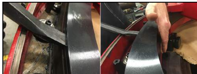
FIGURE 5-6. CHECKING FOR PLAY BETWEEN THE TRACK RING AND THE STATIONARY RING
