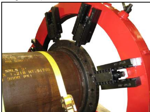
FIGURE 2-1. EXTENSION FEET INSTALLED
