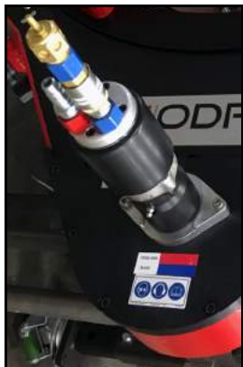
FIGURE 3-14. INSTALLED AIR MOTOR DRIVE
