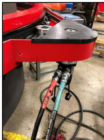
FIGURE 3-15. INSTALLED HYDRAULIC MOTOR DRIVE (BOTTOM SIDE)
