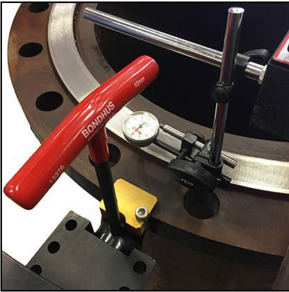
FIGURE 3-8. DIAL INDICATOR MOUNTED FOR LEVELING
