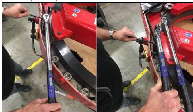
FIGURE 5-5. ADJUSTING AND TIGHTENING OF THE BUSHINGS AND CAP SCREWS
