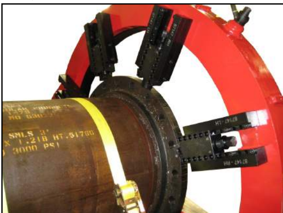
FIGURE 2-1. EXTENSION FEET INSTALLED
