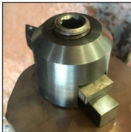
FIGURE 3-10. .50" TOOL ADAPTER INSTALLED (P/N 89175)
