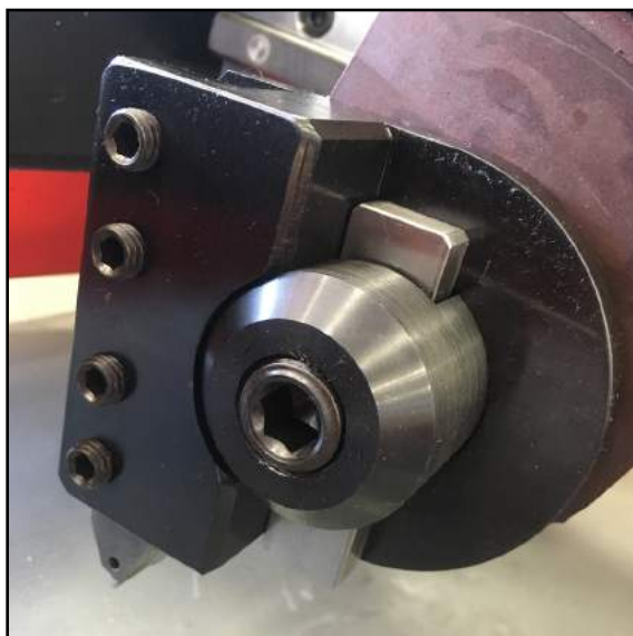
FIGURE 3-11. OFFSET TOOL HOLDER (P/N 89203)
