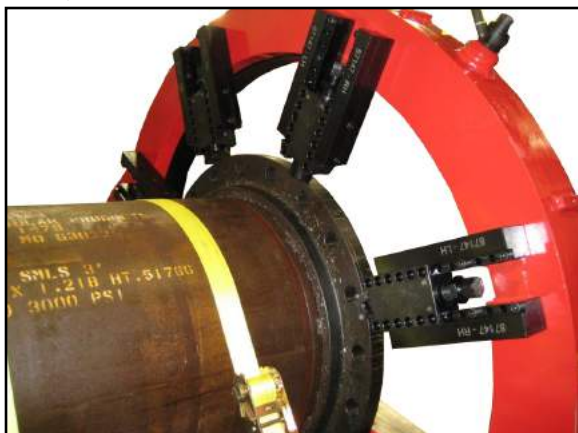
FIGURE 2-1. EXTENSION FEET INSTALLED
