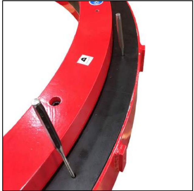
FIGURE 5-3. PUNCHES USED FOR GUARD INSTALLATION
