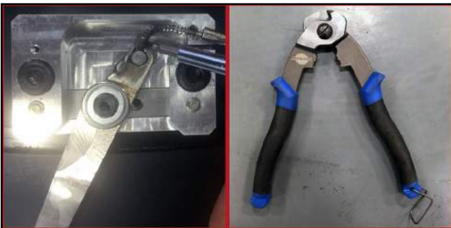
FIGURE 5-8. BARREL END OF CABLE REMOVAL (LEFT); CABLE AND HOUSING CUTTERS (RIGHT)
