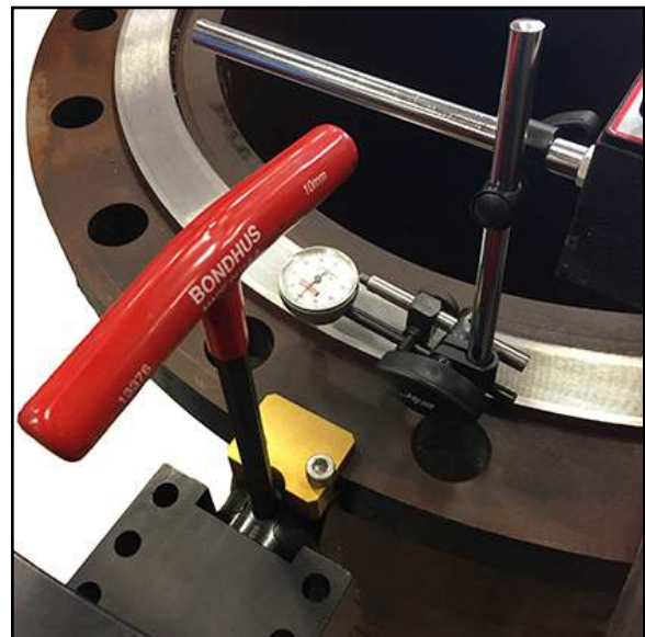
FIGURE 3-8. DIAL INDICATOR MOUNTED FOR LEVELING
