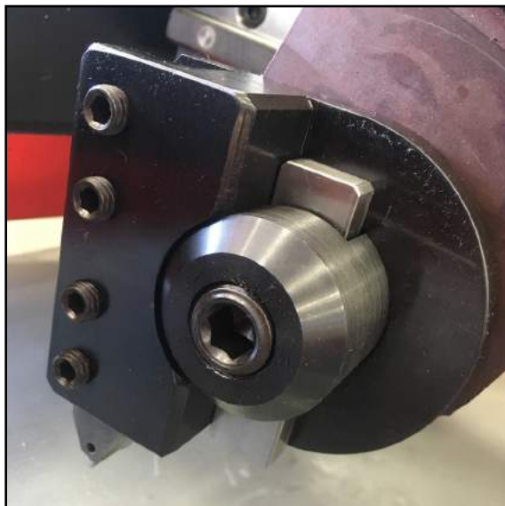
FIGURE 3-11. OFFSET TOOL HOLDER (P/N 89203)
