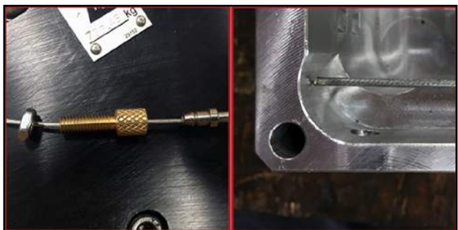
FIGURE 5-10. 90° ELBOW, ADJUSTING NUT AND JAM NUT (LEFT); CABLE END SHOWN AT TRIMMING LOCATION (RIGHT)
