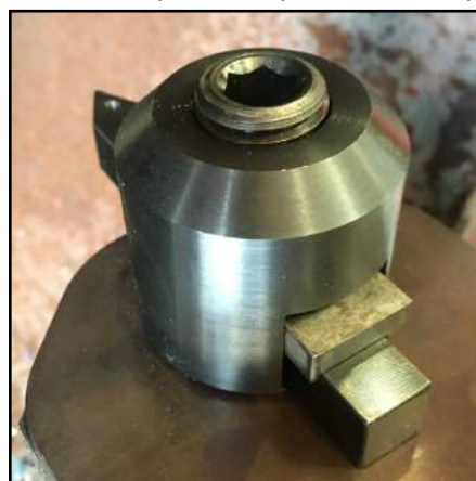
FIGURE 3-10. .50" TOOL ADAPTER INSTALLED (P/N 89175)
