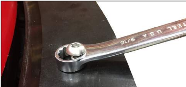
FIGURE 5-2. BOX WRENCH OVER SCREW
