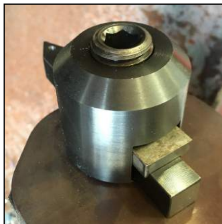
FIGURE 3-10. .50" TOOL ADAPTER INSTALLED (P/N 89175)
