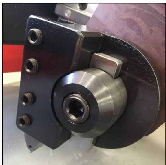
FIGURE 3-11. OFFSET TOOL HOLDER (P/N 89203)
