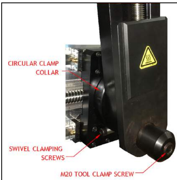
FIGURE 3-9. LOCATION OF SWIVEL CLAMPING SCREW
