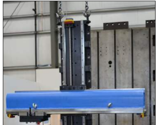
Example of Vertical Lifting
