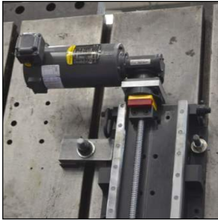
Motor attached to ballscrew on bed
