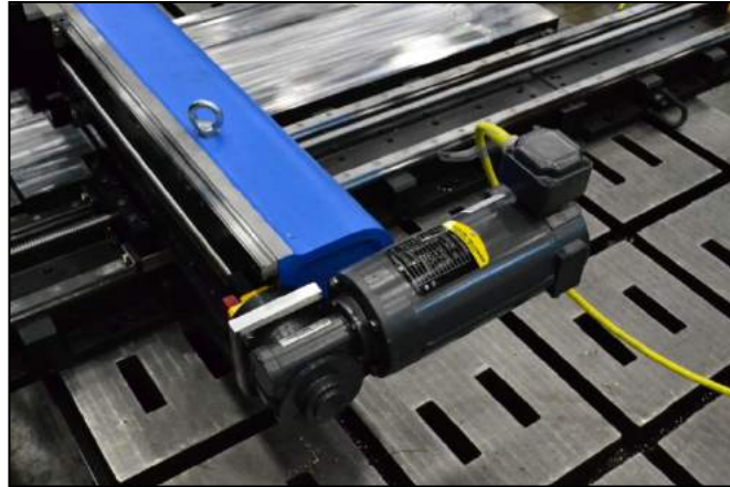
Motor attached to ballscrew on ram
