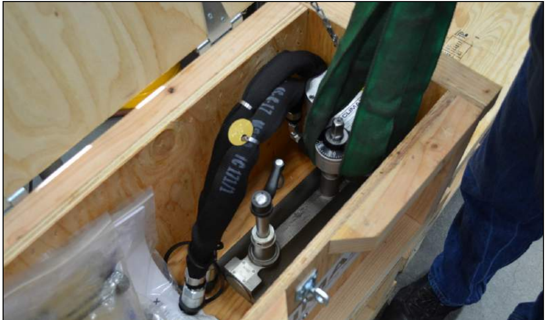
FIGURE 3-1. LIFTING FROM THE CRATE USING A STRAP
