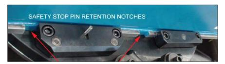
FIGURE 3-17. SAFETY STOP PIN RETENTION NOTCHES
