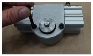
FIGURE 3-31. DETAIL OF FEED SHAFT BOLTS
