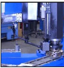
FIGURE 3-56. DIAL INDICATOR INSTALLED
