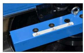
FIGURE 3-21. COUNTERWEIGHT FASTENERS
