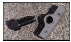
FIGURE 3-3. SAFETY WELD PLATES
