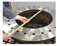
Set machine onto flange using setup fingers. Lightly tighten leveling
