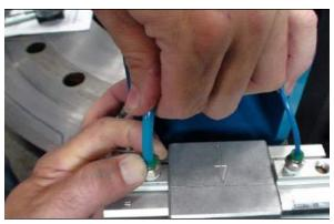
FIGURE 3-34. DISCONNECTING FEED HOSES
