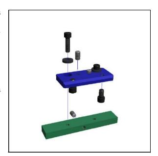
FIGURE 3-38. ATTACHING TACK WELD PLATE
