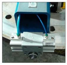
FIGURE 3-30. FEED BOX AIR SUPPLY LINES
