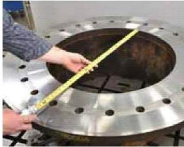
**5** Set machine onto flange using setup fingers. Lightly tighten leveling
