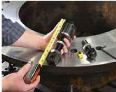
**6** Extend feet into flange. Indicate, level and tighten leveling feet and stationary feet.
