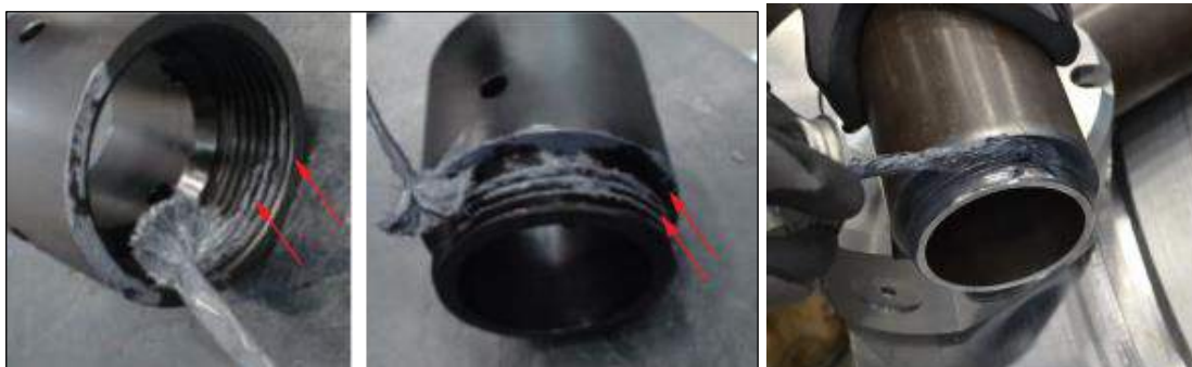
Figure 12. Anti-seize lubricant locations
