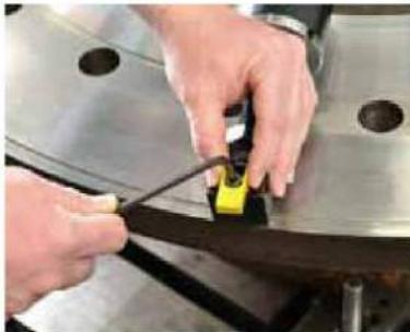
**7** Install tool bit. Connect to power.
