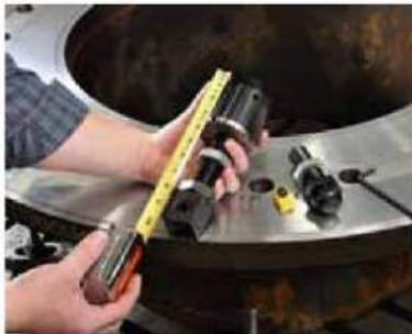
**6** Extend feet into flange. Indicate, level and tighten leveling feet and stationary feet.
