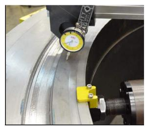
FIGURE 3-6. LEVEL AND CENTER THE ID CHUCK
