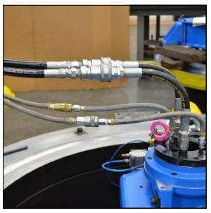
FIGURE 3-8. CONNECT THE HOSES (HYDRAULIC VERSION)
