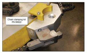
FIGURE 3-23. ATTACHING THE OD MOUNT USING THE CLIMAX CHAIN CLAMP KIT
