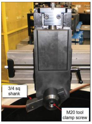
FIGURE 3-30. DETAIL OF TOOL HOLDER
