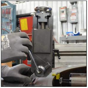
FIGURE 3-7. INSTALL A TOOL BIT
