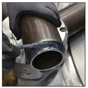
FIGURE 3-12. APPLYING ANTI-SEIZE COMPOUND
