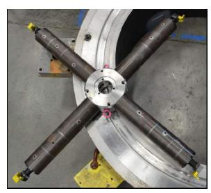
FIGURE 3-3. ASSEMBLE THE ID CHUCK
