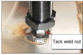
FIGURE 3-22. ATTACHING THE OD MOUNT WITH A TACK-WELD NUT
