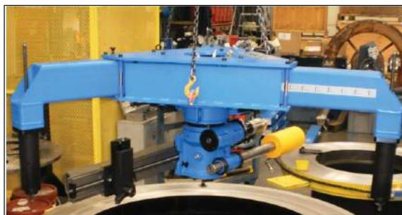
FIGURA 3-19. ENSAMBLAJE DE AMARRE EXTERIOR
