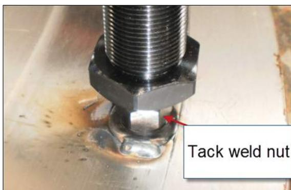
FIGURA 3-22. ACOPLAMIENTO DEL AMARRE EXTERIOR CON UNA TUERCA SOLDADA CON TACHUELAS
