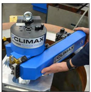
FIGURE 3-10. SLIDING THE MACHINING ARM INTO PLACE
