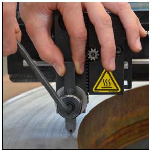
FIGURE 3-20. TOOL BIT INSTALLATION
