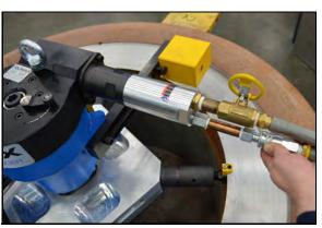
FIGURE 3-23. AIR HOSE CONNECTION
