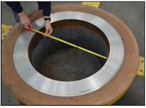
FIGURE 3-3. MEASURING THE BORE DIAMETER
