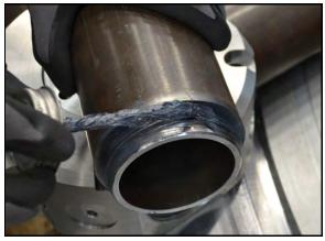
FIGURE 3-5. APPLYING ANTI-SEIZE COMPOUND
