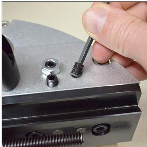
**FIGURE 3-34. RETIRER LE BOUCHON FILETÉ (FF1200 ILLUSTRÉE)**
