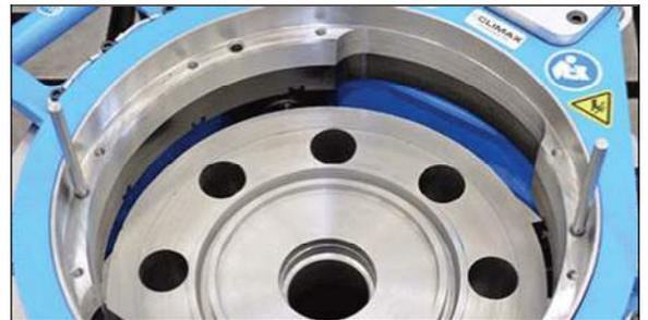
**FIGURE 3-18 - TIGES DE 0,3125 PO (7,9375 MM) POUR FAIRE TOURNER MANUELLEMENT LES ROULEMENTS DE L'UNITÉ D'ENTRAÎNEMENT ROTATIF (RDU) ROULEMENT (FF1200 ILLUSTRÉE)**
