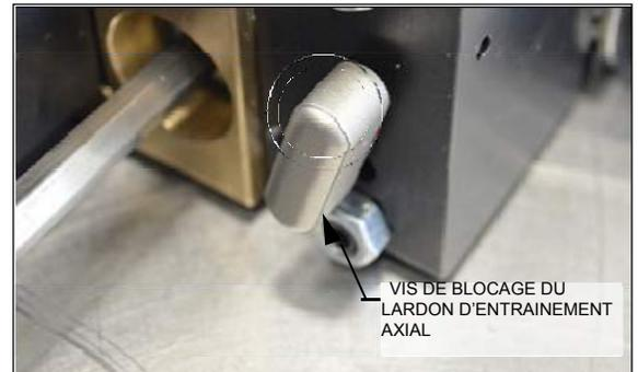
**FIGURE 4-3. VIS DE BLOCAGE DU LARDON D'ENTRAINEMENT AXIAL (FF1200 ILLUSTRÉE)**
