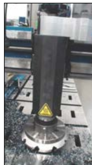
FIGURE 3-22. INSTALLED MILLING HEAD
