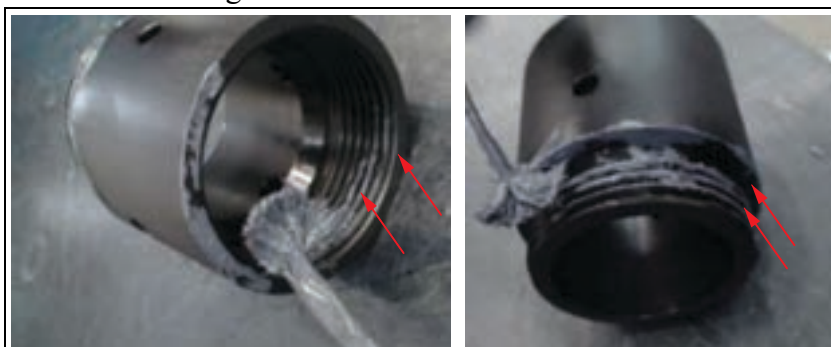
FIGURE 3-12. LOCATIONS TO APPLY ANTI-SEIZE
