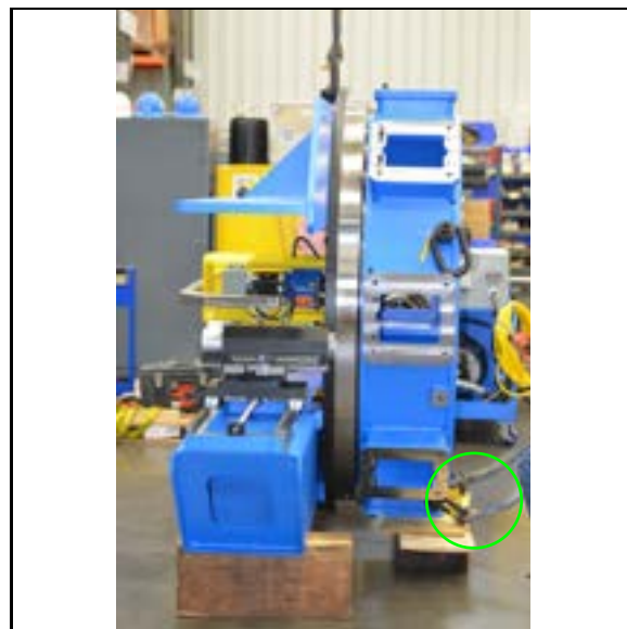
FIGURE 3-30. VERTICAL CM6200 ON BLOCKS WITH STRAPS RE-ATTACHED
