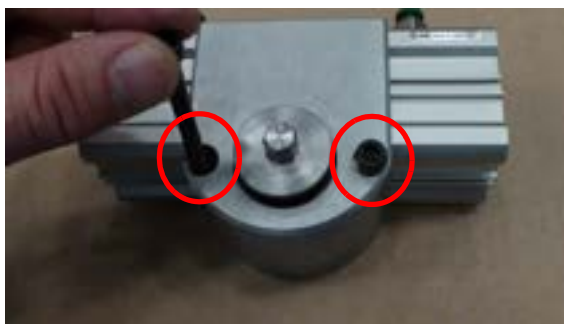
FIGURE 4-44. REMOVAL OF BOLTS TO REVERSE FEED DIRECTION
