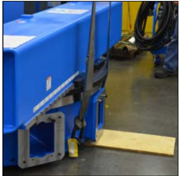
FIGURE 3-28. PLYWOOD AND STRAPS FOR INVERSION
