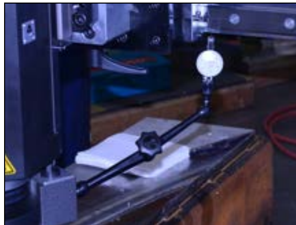
FIGURE 4-4. SPINDLE ROTATED TO THE RAM SURFACE
