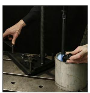
FIGURE 3-21. PARALLELISM CHECK AT 6 O'CLOCK
