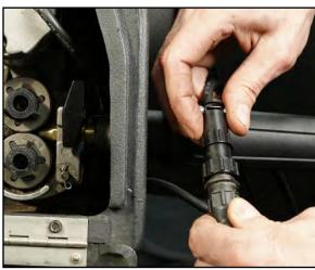
FIGURE 3-27. WIRE FEED CONTROL CABLE CONNECTED TO THE WIRE FEEDER
