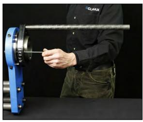
FIGURE 3-4. TIGHTENING THE SET SCREWS
