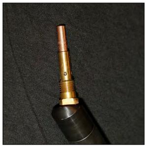
FIGURE 3-10. LINER THROUGH DIFFUSER GAS HOLES
