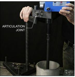
FIGURE 3-22. BW2600 ARTICULATED AT THE BORE CENTER (ARTICULATION JOINT SHOWN)
