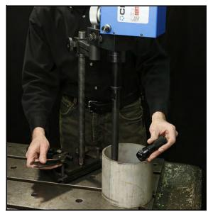
FIGURE 3-20. PARALLELISM CHECK AT 3 O'CLOCK
