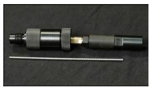
FIGURE 3-30. LINER AND STANDARD TORCH ADAPTER
