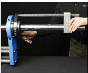
FIGURE 3-3. ALIGNMENT TOOL OVER THE MOUNTING ROD
