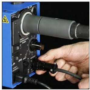
FIGURE 3-25. WIRE FEED CONTROL CABLE CONNECTED
