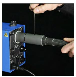
FIGURE 3-24. WIRE FEED CONDUIT CONNECTED
