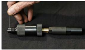
FIGURE 3-31. LINER TIGHTENED IN THE SWIVEL
