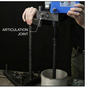
FIGURE 3-22. BW2600 ARTICULATED AT THE BORE CENTER (ARTICULATION JOINT SHOWN)
