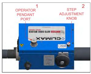
FIGURE 4-2. LOCATION OF THE STEP ADJUSTMENT KNOB
