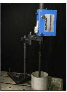
FIGURE 3-19. BW2600 ON THE MOUNTING ROD
