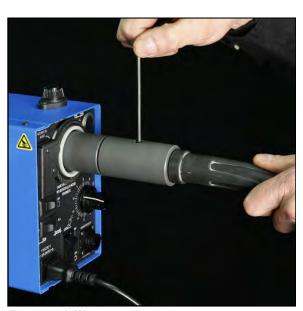
FIGURE 3-24. WIRE FEED CONDUIT CONNECTED
