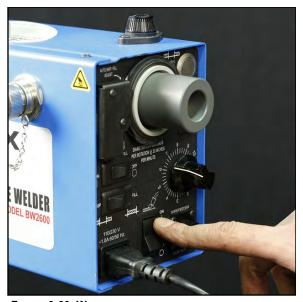
FIGURE 3-29. WELD START SWITCH
