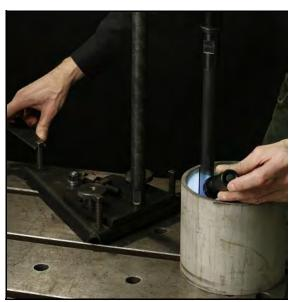
FIGURE 3-21. PARALLELISM CHECK AT 6 O'CLOCK
