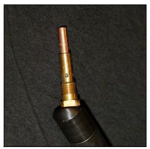
FIGURE 3-10. LINER THROUGH DIFFUSER GAS HOLES
