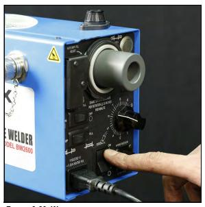
FIGURE 3-29. WELD START SWITCH
