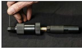
FIGURE 3-31. LINER TIGHTENED IN THE SWIVEL
