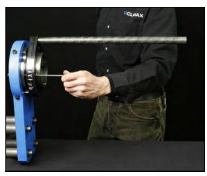
FIGURE 3-4. TIGHTENING THE SET SCREWS
