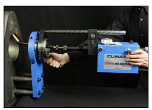
FIGURE 3-16. SUPPORTING THE BORE WELDER FOR SAG ADJUSTMENT (EXTENSIONS NOT SHOWN)
