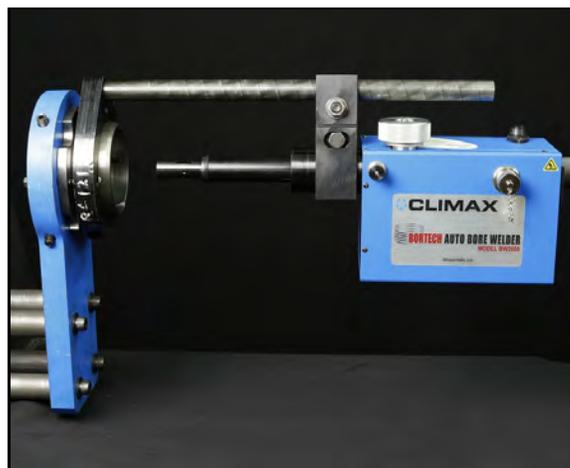
**FIGURA 3-6. BW2600 Y MONTAJE RADIAL EN VARILLA DE MONTAJE**
