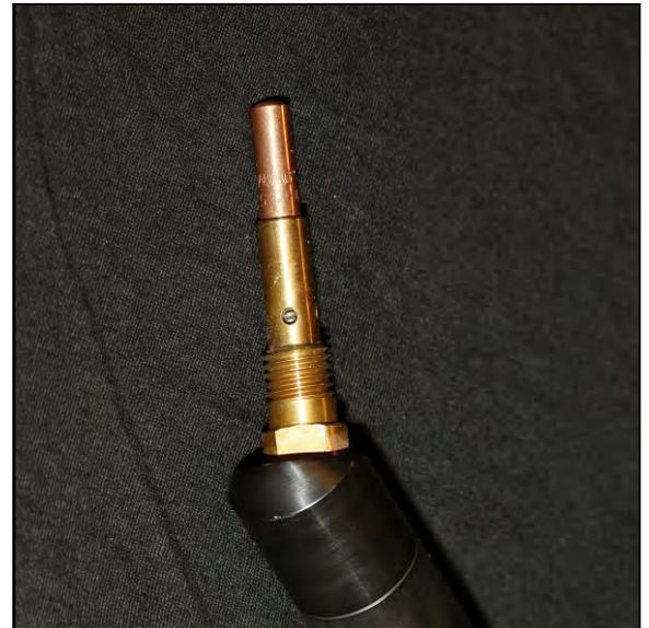
FIGURE 3-10. GAINE VISIBLE AU TRAVERS DES TROUS DU DIFFUSEUR DE GAZ
