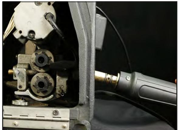
FIGURE 3-26. CONNEXION DU CONDUIT D'APPORT DE FIL
