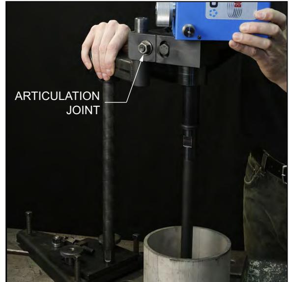
FIGURE 3-22. BW2600 ARTICULÉE AU CENTRE DE L'ALÉSAGE (JOINT D'ARTICULATION ILLUSTRÉ)
