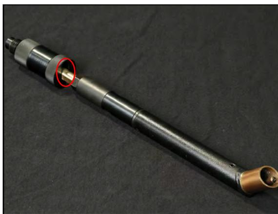
FIGURE 3-32. ORIENTATION DE LA BUSE DE TORCHE
