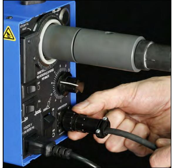
FIGURE 3-25. CÂBLE DE COMMANDE DU DÉVIDOIR BRANCHÉ
