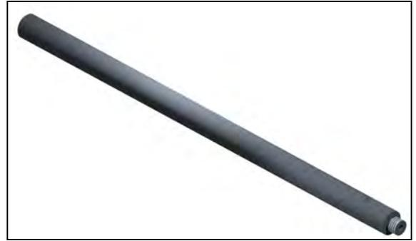
FIGURE 2-12. DÉTAIL DE LA TIGE DE MONTAGE RÉF. 30773
