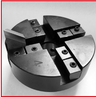
FIGURE 3-8. SLIDING TOOL HOLDER WITH CUTTING BIT.
