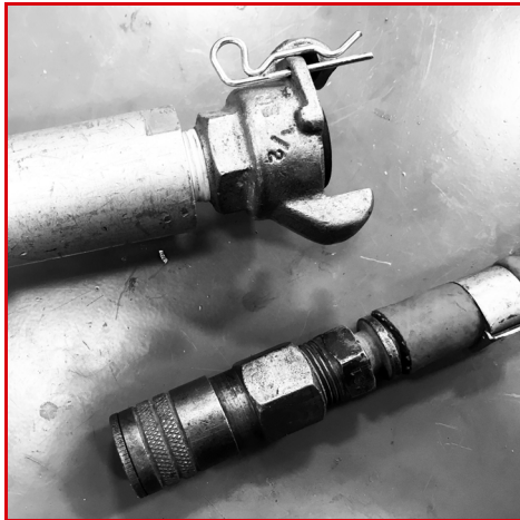
FIGURE 3-10. UNIVERSAL COUPLER (TOP) AND QUICK DISCONNECT (BOTTOM)
