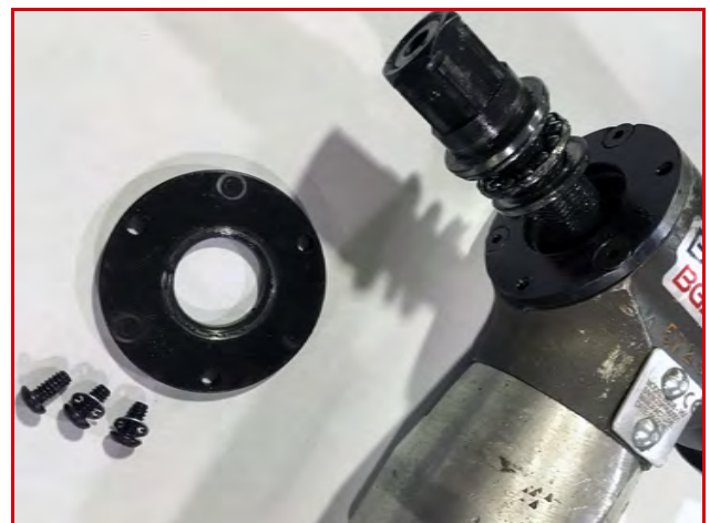
FIGURE 3-4. CHANGING THE CENTER SHAFT
