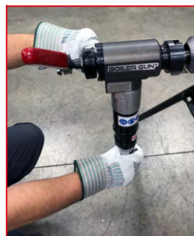
FIGURE 4-1. HAND POSITIONING DURING BOILER GUN OPERATION
