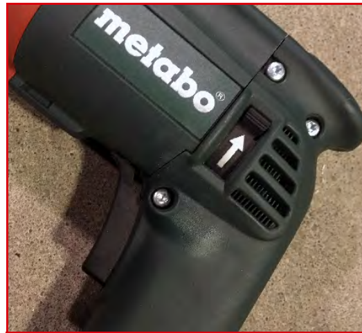
FIGURE 3-10. MOTOR DIRECTION CONTROL SET TO FORWARD
