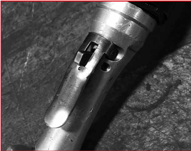
FIGURE 2-2. PNEUMATIC MOTOR THROTTLE LEVER
