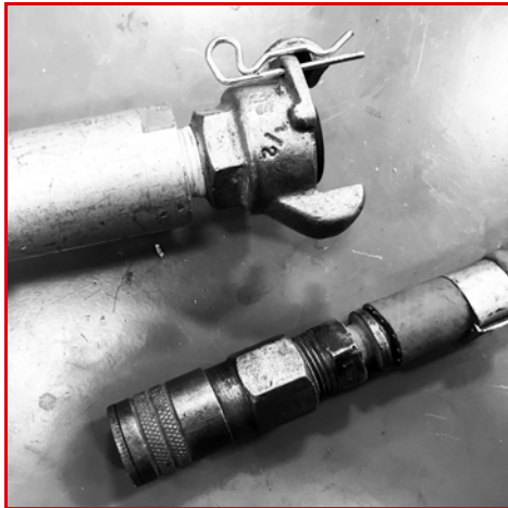
FIGURE 3-9. UNIVERSAL COUPLER (TOP) AND QUICK DISCONNECT (BOTTOM)
