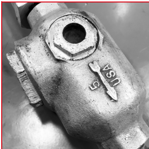
FIGURE 5-1. IN-LINE OILER SIGHT GLASS
