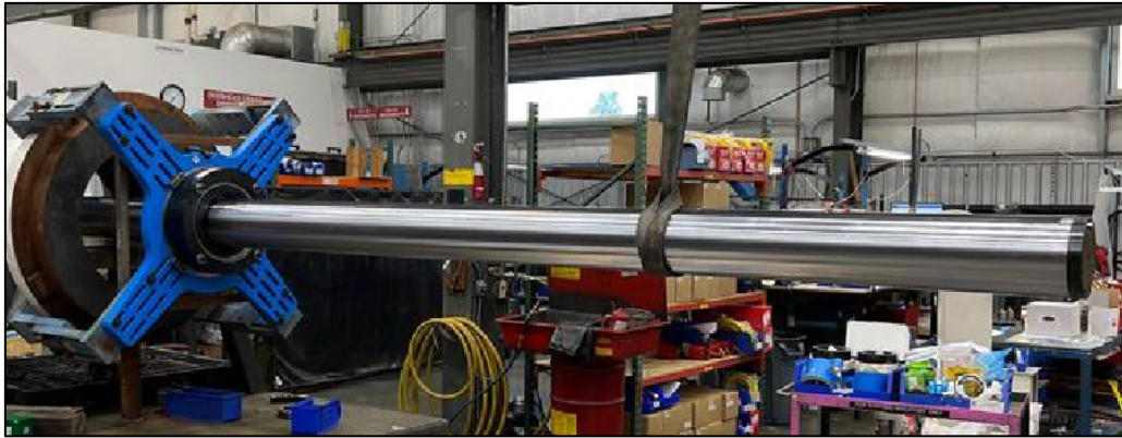
Figure 15. Boring bar into the bearings
