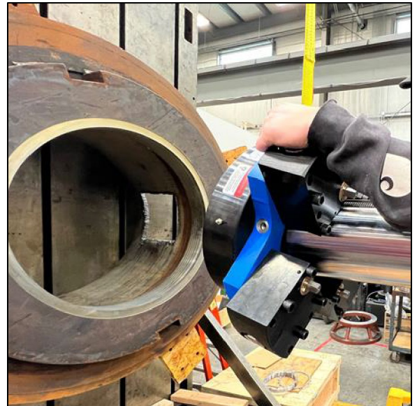
Figure 19. Positioning the bearing support assembly on the bar
