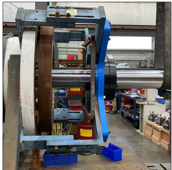
Figure 14. Centering and aligning the bar
