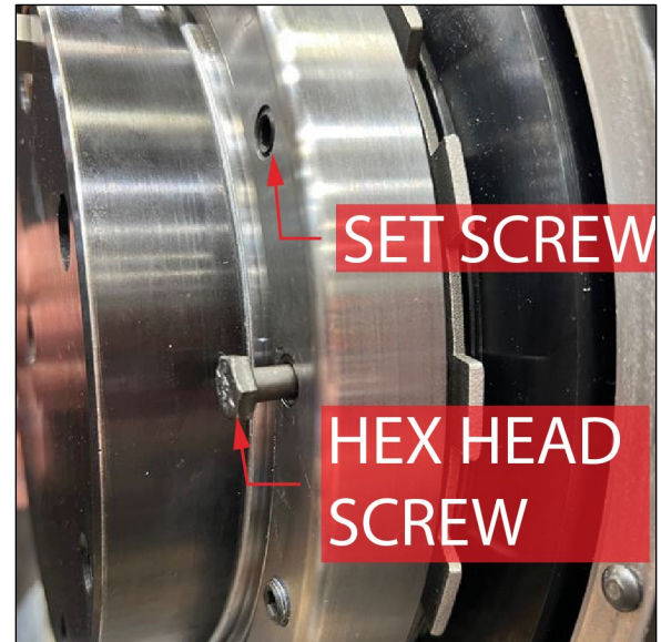
Figure 16. Set screw and hex head screw
