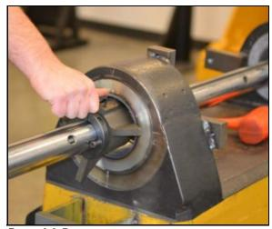
FIGURE 3-2. BORING BAR INSERTION
