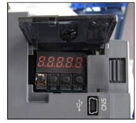
FIGURE D-1. SERVO AMP FUNCTION KEYS
