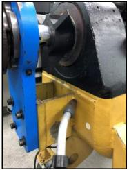
FIGURE 3-4. CENTERING THE SPHERI-CAL BEARINGS
