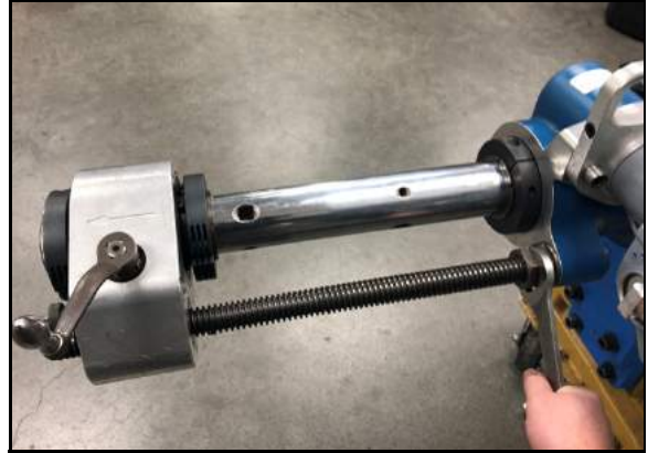
FIGURE 3-10. POSITIONING THE AFU
