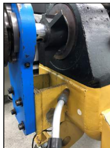
FIGURE 3-4. CENTERING THE SPHERICAL BEARINGS
