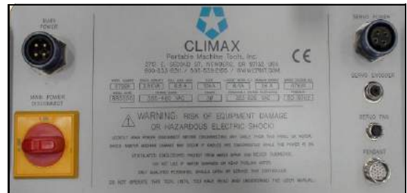
FIGURE 3-15. SERVO MOTOR MAIN CONTROL PANEL
