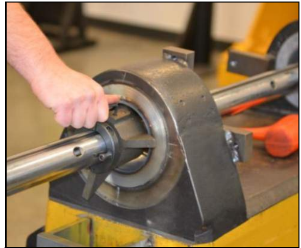
FIGURE 3-2. BORING BAR INSERTION
