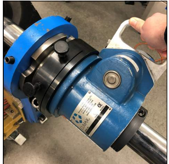
FIGURE 3-9. POSITIONING THE RDU
