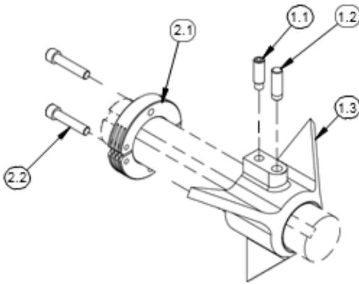
**SET CONES SETUP 2 TO 6 DIA 1-3/4 KEYED BAR**
