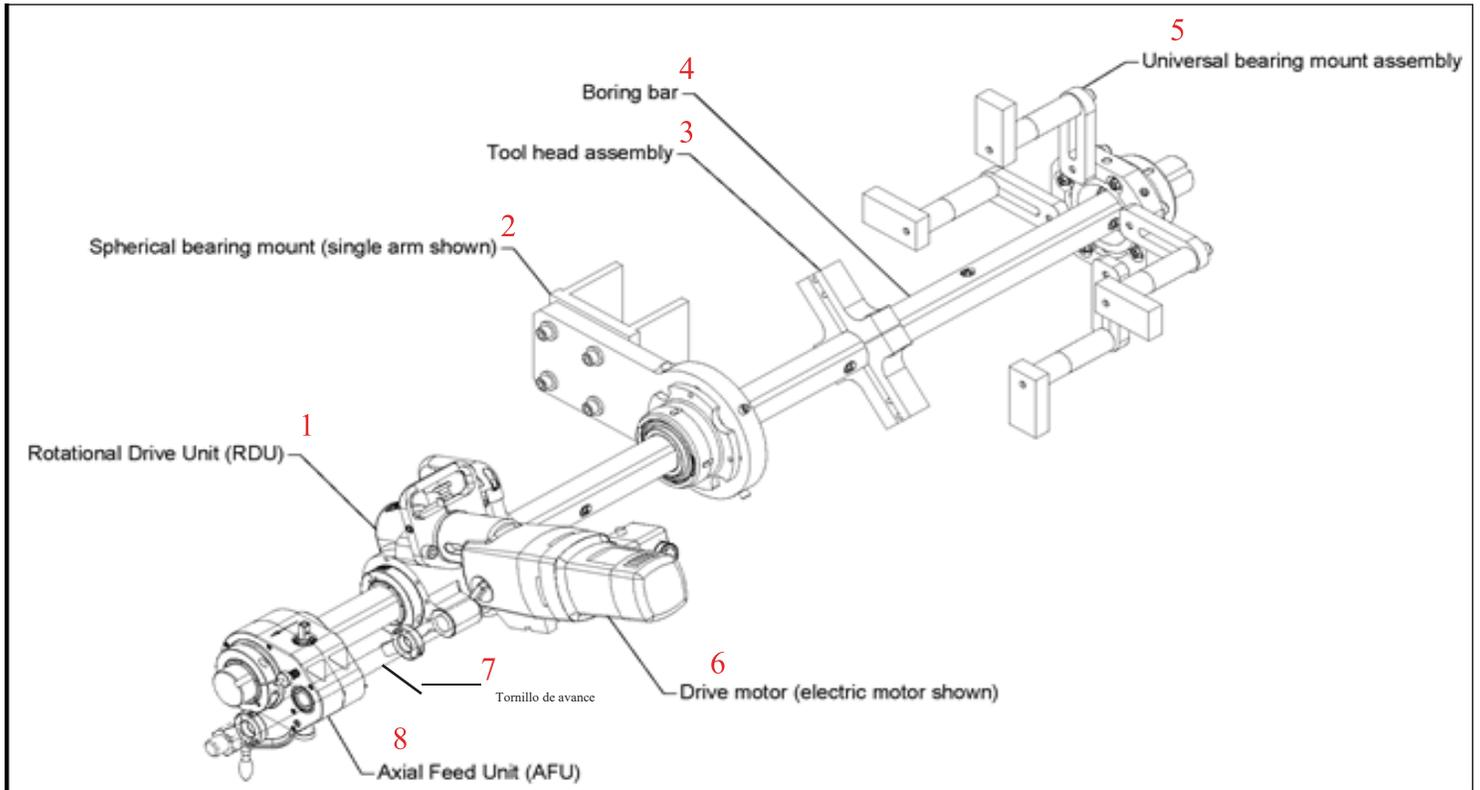
FIGURA 2-1. COMPONENTES BB4500-BB5000 CON MOTOR EIBENSTOCK (SE MUESTRA BB5000)
