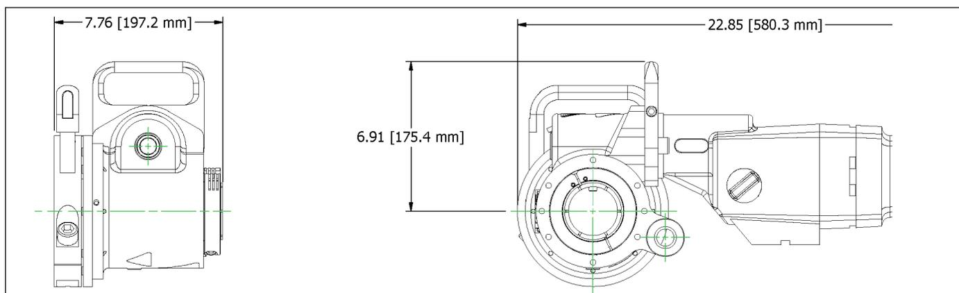
**FIGURA 2-10. DIMENSIONES DEL MOTOR EIBENSTOCK Y DE LA RDU**
