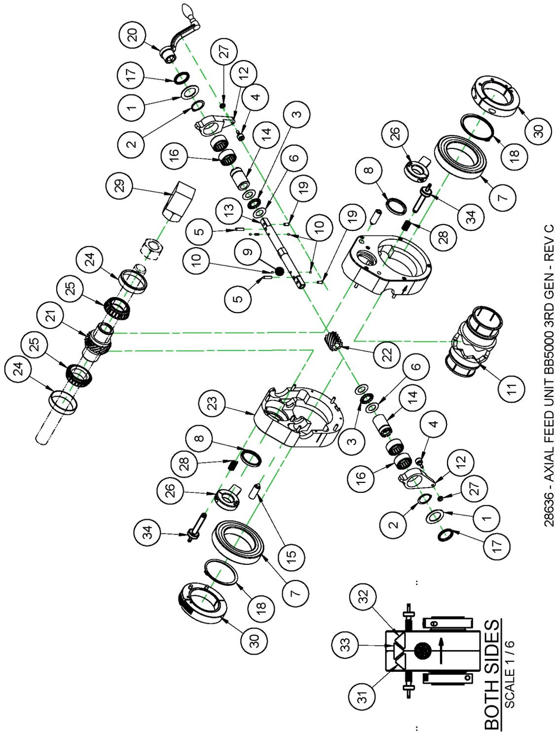
28636 - AXIAL FEED UNIT BB5000 3RD GEN - REV C
