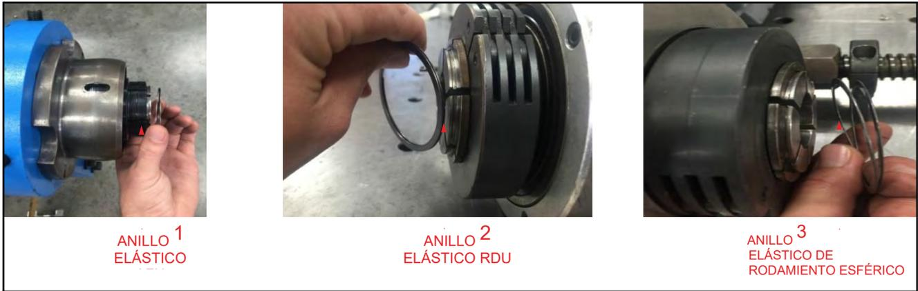
**FIGURA 3-22. REEMPLAZAR ANILLO ELÁSTICO**
