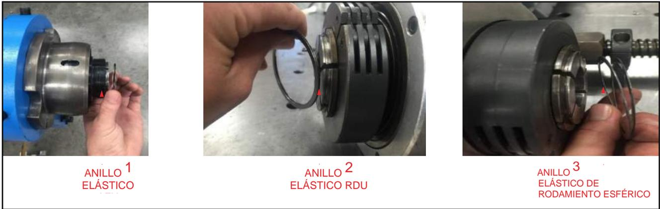
**FIGURA 3-22. REEMPLAZAR ANILLO ELÁSTICO**
