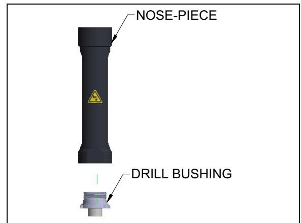
FIGURE 3-3. INSTALLING THE NOSE PIECE BUSHING
