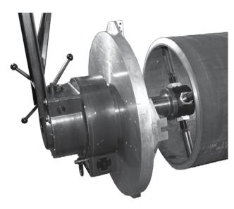
The Miter Mandrel for the MFT-HD has been engineered to center and lock the tool in a minimum of pipe depth. It is especially useful for, but not limited to, elbows.
