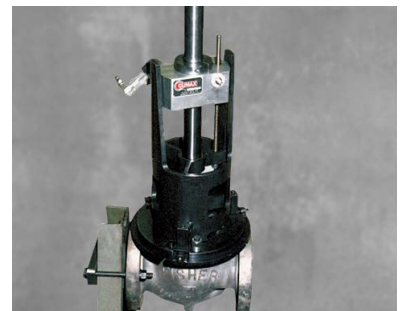
VM8000 Globe and Control Valve Repair
