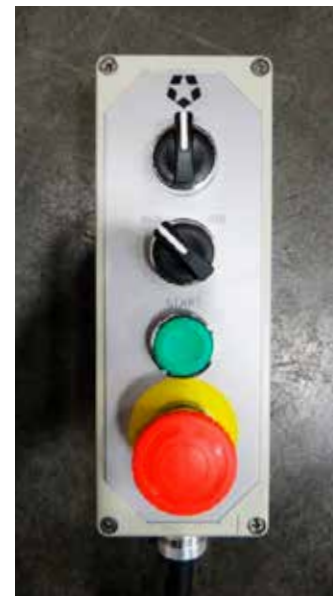
4 Function Pendant with replaceable cordset
